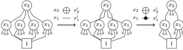
Fig. 5: Effects of applying Toffoli gates to 1:1DDs
