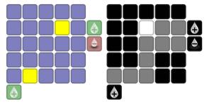
Fig. 8: Left: Information can be shown for the current state – droplets are hidden to emphasize actuation, indicated via yellow-marked cells. Right: Aggregated information – amount of cell actuation on a color scale from black to white.
