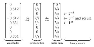
Fig. 3. Biased random selection via binary search on a prefix array. The precomputation in (a) is performed once to facilitate efficient repeated sampling in (b).
