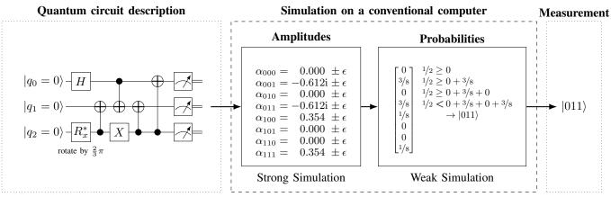
Fig. 2. Mimicking a physical quantum computer by generating individual output samples after strong simulation
