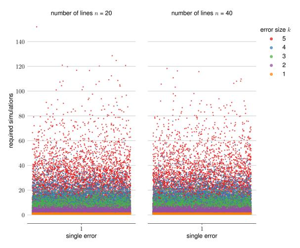
Fig. 8. Confirmation of theoretical results: Scatter-plot of required simulations (y-axis) for detecting a single reversible error of size k in a circuit with n=20 (left plot) and n=40 (right plot) lines. Different colors denote varying values of  $k \in \{1,2,3,4,5\}$ . This experimentally confirms that the distribution of simulations does not depend on the number of lines and that the number of required simulations grows exponentially with the size of the error.
