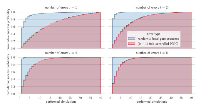
Fig. 9. Comparison of worst-case and average-case errors: performed simulations (x-axis) vs. cumulative distribution function (cdf) for detecting l=1,2,4,6 reversible errors of size k=5 (y-axis). The red curve corresponds to injecting worst-case errors, while the blue curve delineates the cdf for detecting randomly generated errors of the same size. This goes to show, that average-case errors require far less simulations than worst-case ones.
