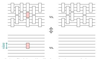
Fig. 2. Illustration of main rigorous contributions: Simulations with uniformly random inputs completely expose any single reversible error in a given reversible circuit. The two scenarios are exactly equivalent ("no masking"). In the lower scenario, the probability of correct distinction is governed by the size k of the error, not the total number of lines.
