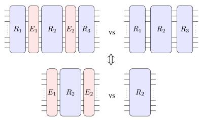
Fig. 5. Partial simplification for multiple errors: Simulation with uniformly random inputs exposes multiple errors only partially. Everything before the first error  $(R_1)$  and after the last error  $(R_3)$  can be safely ignored, but the part in between  $(R_2)$  does matter. Different circuit structures can lead to strikingly different error detection probabilities.
